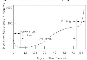
Figure 5. Insulation Resistance vs. Drying Time.
